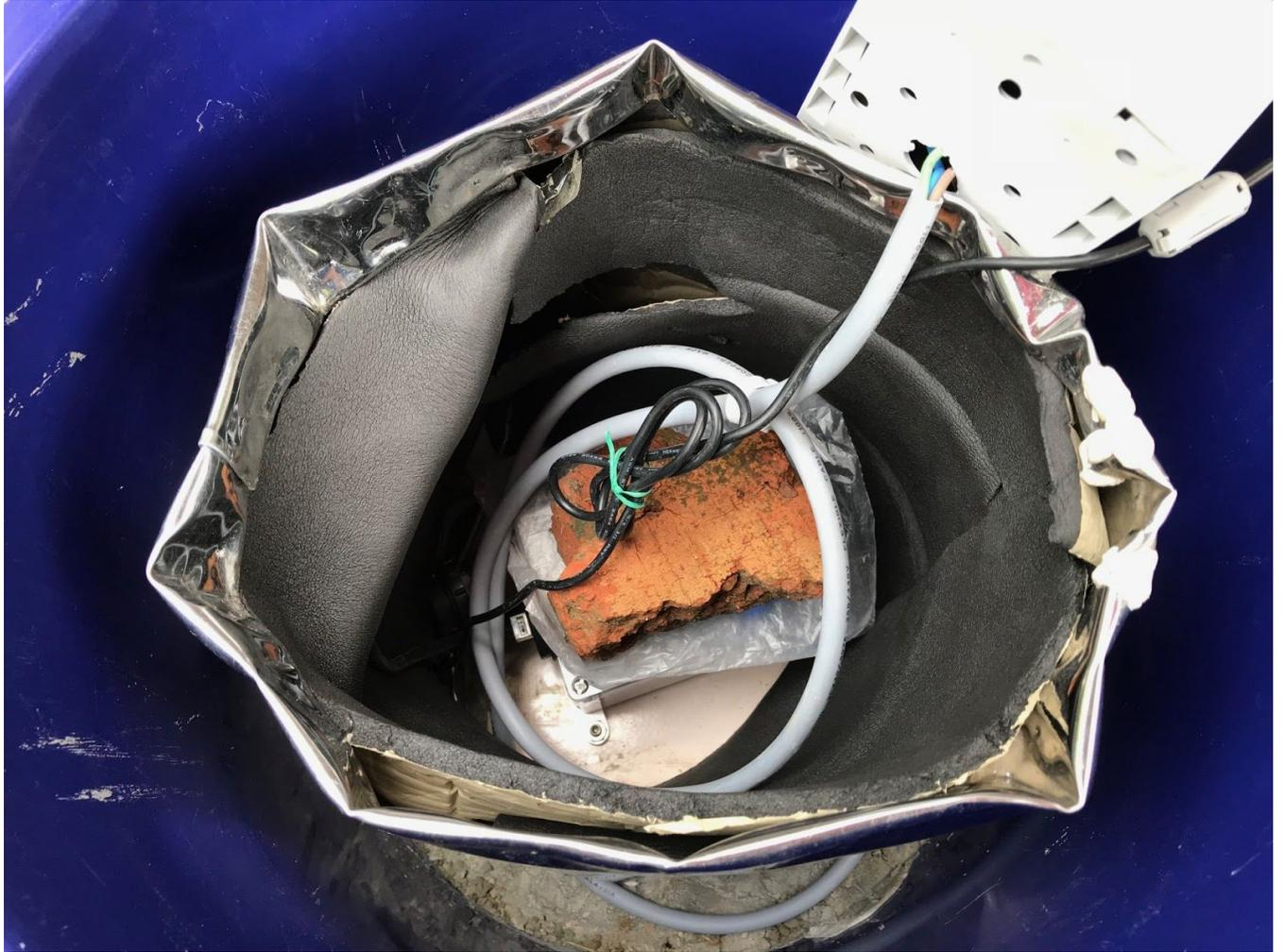
After securing the stainless steel bin with blu tac and placing in some insulating material inside the bin, a brick is placed on top of the RS4D to keep it in place.
