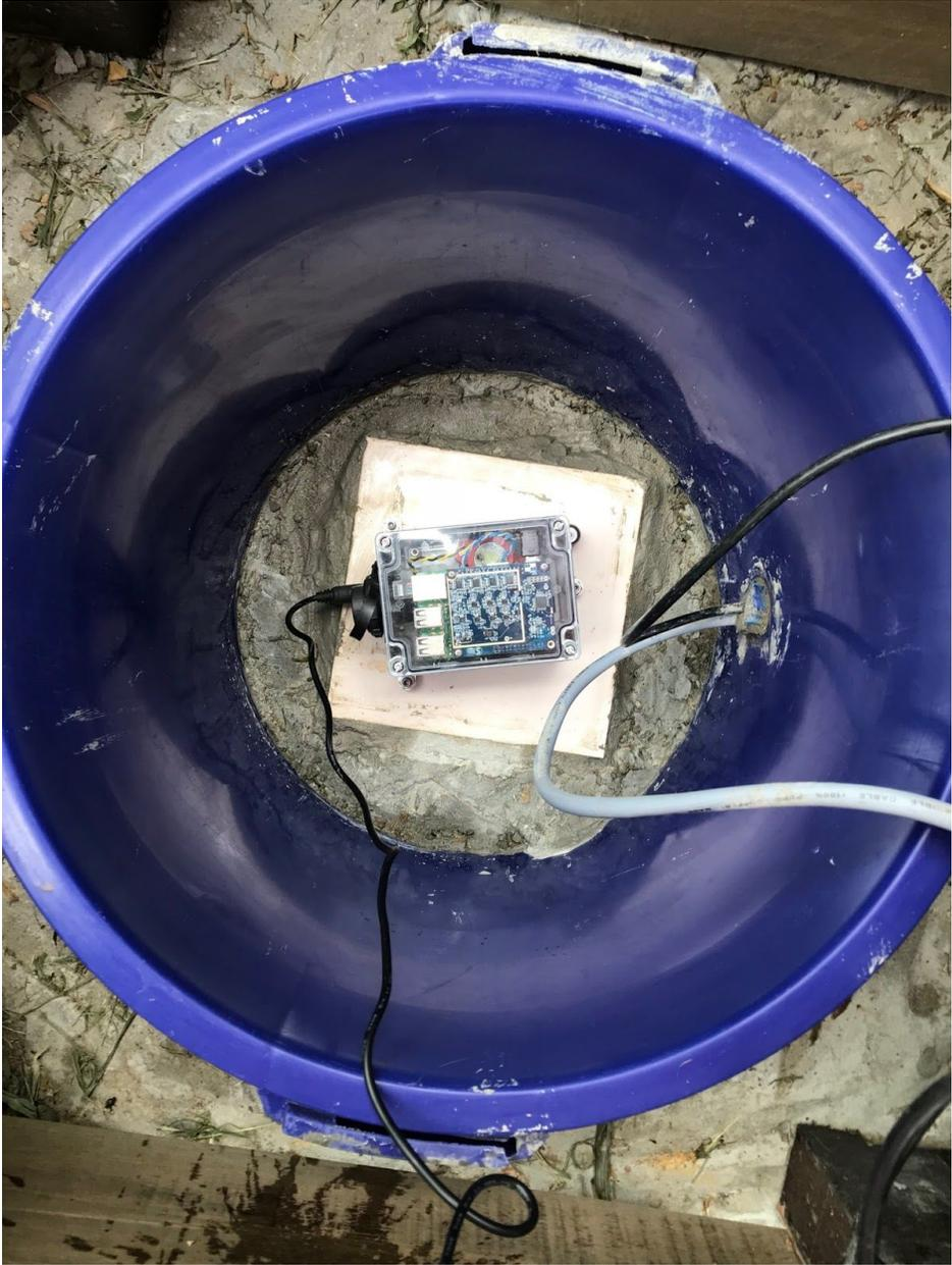
18/09/02 - 2 days after tile placement, the AM.RA82A RS4D is inside the vault. Checking device position and leveling. It is in the all weather enclosure.
